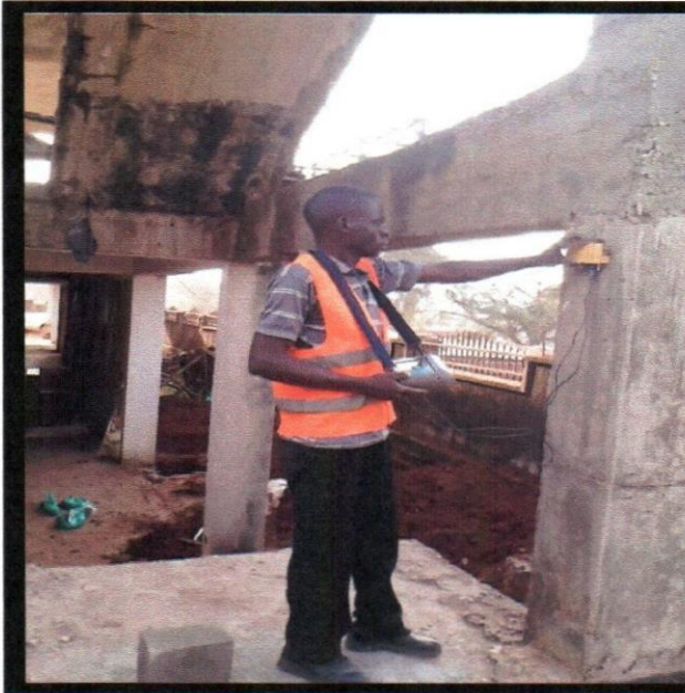
Cover meter survey Test indicates position of reinforcement bars in hardened concrete
