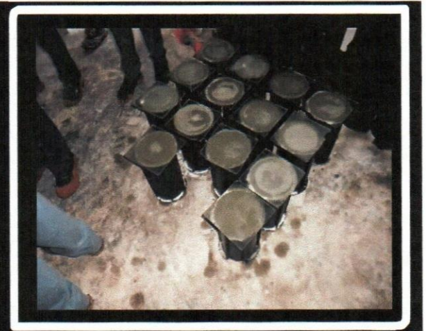
Preparation of concrete cylindrical samples for compressive strength Test.
