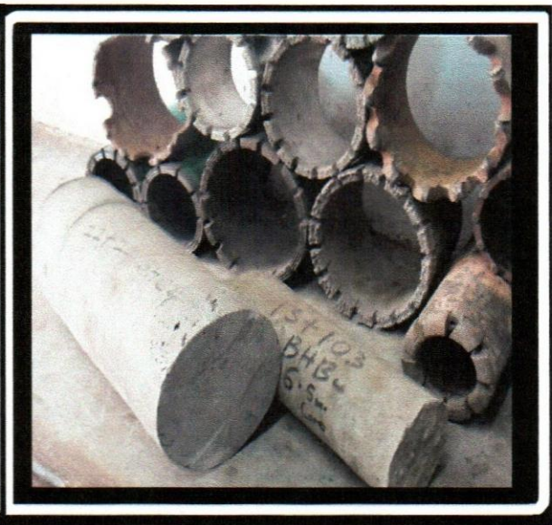
Core Drilling bits for rock sampling
